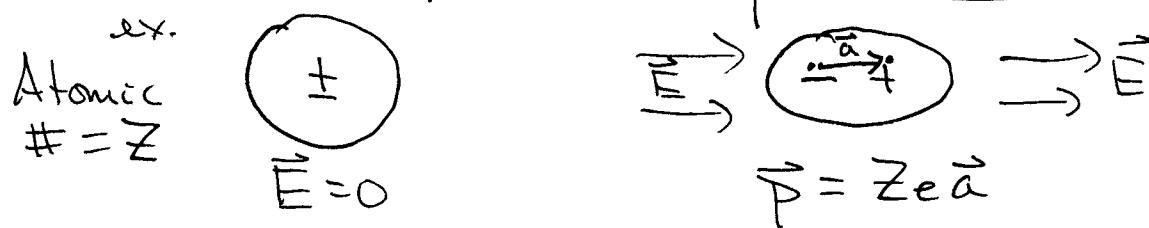
$$\text{Polarization Vector} = \vec{P} \equiv N \vec{p} = \frac{\text{dipole moment}}{\text{Volume}}$$
