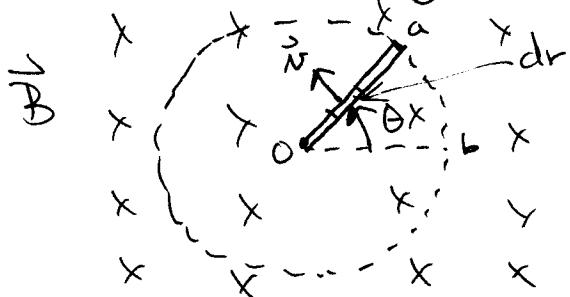
A motional emf  $dE$  develops across element  $dr$  of the rod as it moves with velocity  $v$ .
