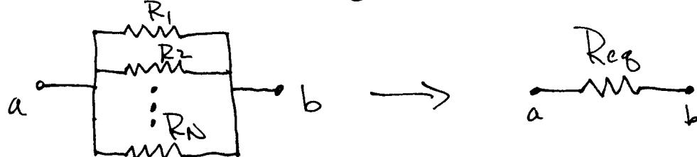
II F 1)  $\frac{1}{R_{\text{eq}}} = \sum_{i=1}^{N_f} \frac{1}{R_i} = \frac{1}{R_1} + \frac{1}{R_2} + \dots + \frac{1}{R_N}$
