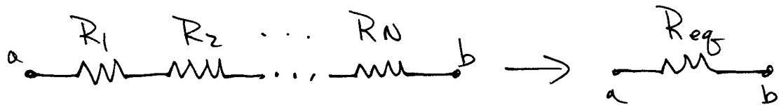
$$R_{\text{eq}} = \sum_{i=1}^{N_f} R_i = R_1 + R_2 + \dots + R_N$$
