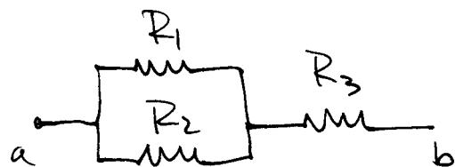
$$R_{12} = \frac{R_1 R_2}{R_1 + R_2}$$
