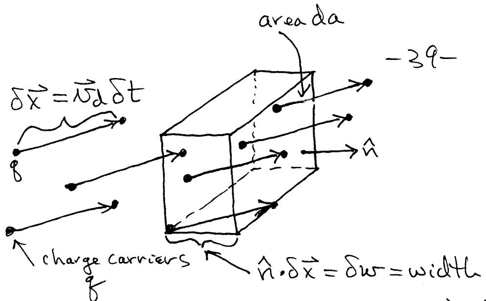
In time  $\delta t$ , each charge carrier moves  $\delta \vec{x} = \vec{v}_d \delta t$ . Charge  $\delta Q$  passes through area  $da$  in time  $\delta t$
