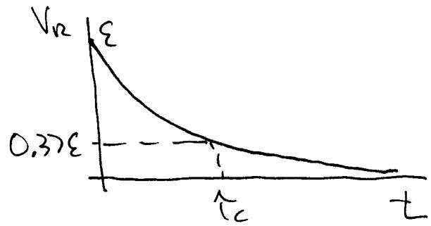
b) Throw switch from a to b: Discharge Capacitor
