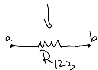
$$\begin{aligned} R_{123} &= R_{12} + R_3 \\ &= \frac{R_1 R_2}{R_1 + R_2} + R_3 \end{aligned}$$
