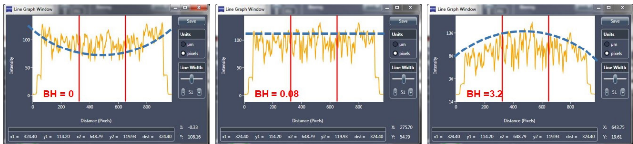
Figure 3-17 Understanding the Beam Hardening Constant Value
