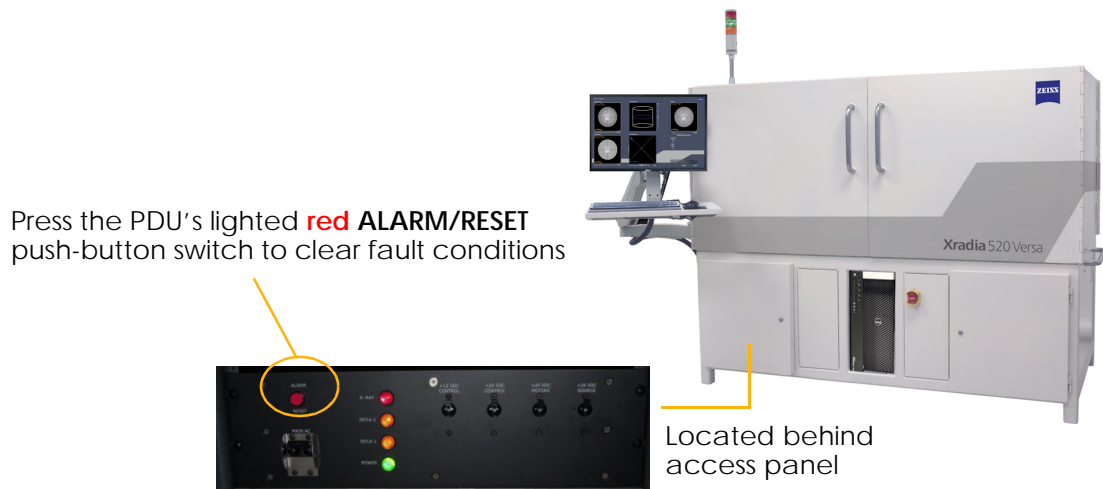
Figure J-2 Press the PDU's Lighted Red ALARM/RESET Push-Button Switch to Clear Fault Conditions (Xradia 520 Versa Shown)
