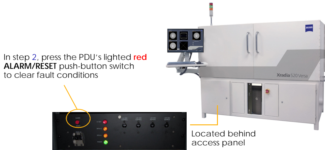
Figure A-2 Press the PDU's Lighted Red ALARM/RESET Push-Button Switch to Restore X-ray Source Power (Xradia 520 Versa Shown)
