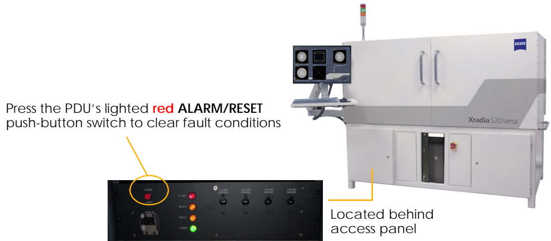
Figure A-8 Press the PDU's Lighted Red ALARM/RESET Push-Button Switch to Clear Fault Conditions (Xradia 520 Versa Shown)
