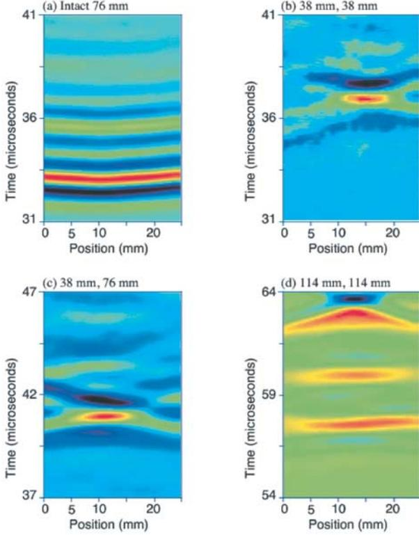
**Figure 2.** Experimental results showing the amplitude (represented by color scale; red-high, blue-low) as a function of time (in microseconds) and position (horizontal axis in millimeters) at 7 MPa. The numbers at the top of each image represent  $d_1$  and  $d_2$ .  $d_1$  represents the distance from the plane of the source to the plane of the fracture, and  $d_2$  represents the distance from the fracture to the plane of the receiver.
