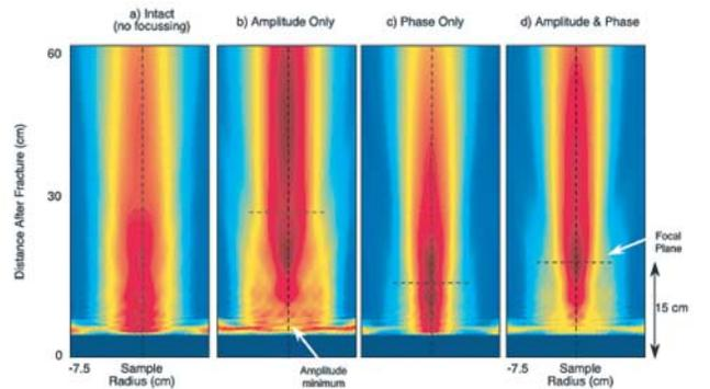
**Figure 3.** Theoretical diffraction results for 0.5 MHz showing (a) an intact sample, (b) the effect of amplitude only, (c) the effect of the phase only, and (d) the complete effect of both amplitude and phase. The wavelength is 1 cm and the fracture specific stiffness at the center is  $1 \times 10^{13}$  [Pa/m].
