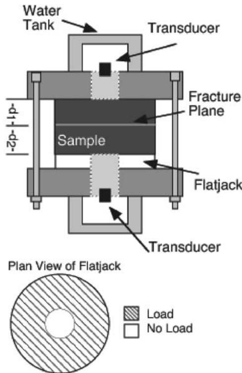
**Figure 1.** A sketch of the wavefront imaging apparatus and plan view of annular load distribution.
