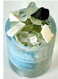
Figure 2 – Sandstone core sample within resin core holder with mineral fragments.
