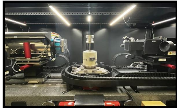
Figure 6: The Deben pictured inside of the Zeiss 3DXRM.
