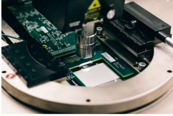
Figure 4 Close-up of the probe station in use [7]
