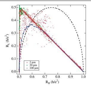
FIG. 2 (color).  $R_L$  vs  $R_H$  for the 2, 20, and 100  $\mu$ m Hall bars in the vicinity of the  $\nu=2$ -1 transition, T=10 mK. Dashed line: the theoretical semicircle relation for a macroscopic sample with the same aspect ratio as our samples.
