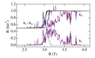
FIG. 4 (color).  $R_L$  and  $R_H$  (purple) and  $R_L + R_H$  (blue) of the 2  $\mu$ m Hall bar, together with  $R_L$  and  $R_H$  (dashed black) and  $R_L + R_H$  (solid black) of the 100  $\mu$ m Hall bar, in the vicinity of the  $\nu = 2$ -1 transition, T = 10 mK. The 100  $\mu$ m traces are shifted to the left by 0.074 T.
