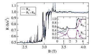
FIG. 3 (color).  $R_{2t}$  and  $R_L + R_H$  of the 2  $\mu$ m Hall bar in the vicinity of the  $\nu=2$ -1 transition, T=10 mK. The  $R_{2t}$  trace is shown after a subtraction of 1402  $\Omega$ . Inset:  $R_L$  and  $R_H$  (purple),  $R_{2t}$  and  $R_L + R_H$  over a wider B range. Note that  $R_L + R_H \neq R_{2t}$  for B < 2 T.
