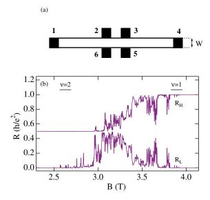
FIG. 1 (color). (a) Geometry of the Hall-bar samples. The black areas represent Au-Ge-Ni contacts. The separation of the current and voltage contacts are  $12 \times W$  and  $2 \times W$ , respectively. (b)  $R_L$  and  $R_H$  vs B of the 2  $\mu$ m Hall bar in the vicinity of the  $\nu = 2$ -1 transition, T = 10 mK.
