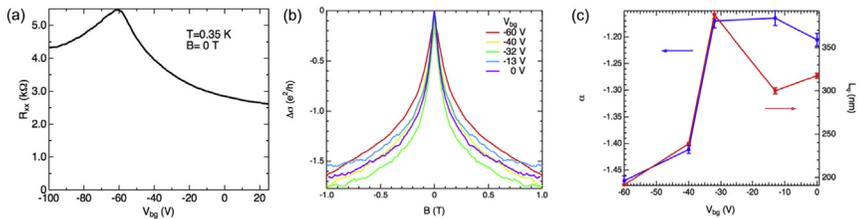
**Figure 7.3** Longitudinal resistance  $R_{xx}$  as a function of the back-gate voltage  $V_{bg}$  at  $T = 0.35$  K and  $B = 0$  T. (b) Magnetoconductance  $\Delta\sigma$  versus magnetic field for various back-gate voltages, marking the weak anti-localisation effect. (c)  $\alpha$  and  $l_\phi$  versus  $V_{bg}$ . All measurements are done in BiSbTeSe<sub>2</sub> flakes obtained by the scotch tape exfoliation from a bulk crystal. Credit: Refs. [22,25].
