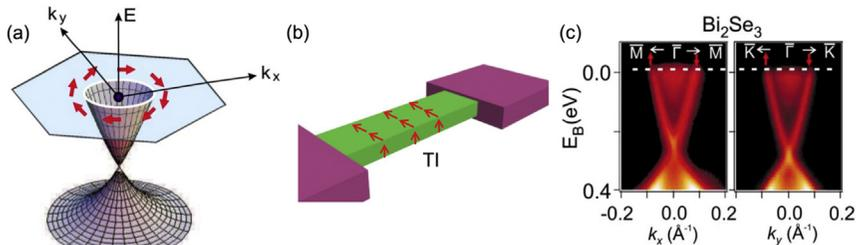
**Figure 7.1** (a) Schematic of spin–helical surface energy dispersion of a typical 3D TI. (b) Schematic of the spin texture in a 3D TI surface state. Spin is always tangential to the surface and perpendicular to the momentum. (c) Band structure of  $\text{Bi}_2\text{Se}_3$  measured by ARPES. Credit: Adapted from Refs. [1,17,42].
