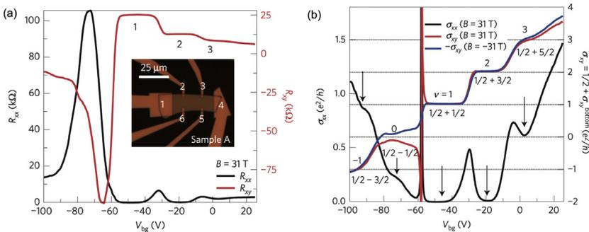
**Figure 7.4** (a) Longitudinal ( $R_{xx}$ ) and Hall ( $R_{xy}$ ) resistance as functions of the back-gate voltage ( $V_{bg}$ ) at  $B = 31$  T and  $T = 0.35$  K. Inset shows the optical image of the device where different electrodes are marked. (b) Calculated 2D longitudinal  $\sigma_{xx}$  and Hall  $\sigma_{xy}$  conductivities from (a). Credit: Ref. [22].
