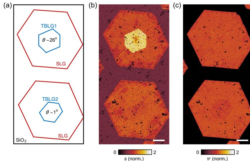
FIG. 2. (a) Sketch of the sample geometry indicating two adjacent TBLG grains with different twist angles with respect to SLG. (b),(c) The near-field images plotting the scattering amplitude ( $s$ ) and phase ( $\psi$ ), respectively. In both images, the amplitude or phase signal is normalized to that of SLG. The laser energy is set to be at  $E = 0.11 \text{ eV}$ . The scale bars represent  $3 \mu\text{m}$ .
