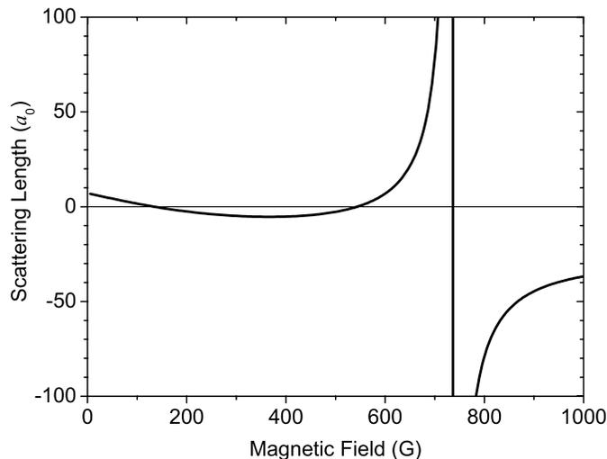
Fig. 1. Coupled-channels calculation of the scattering length for the  $|1,1\rangle$  Feshbach resonance in  ${}^7\text{Li}$ .
