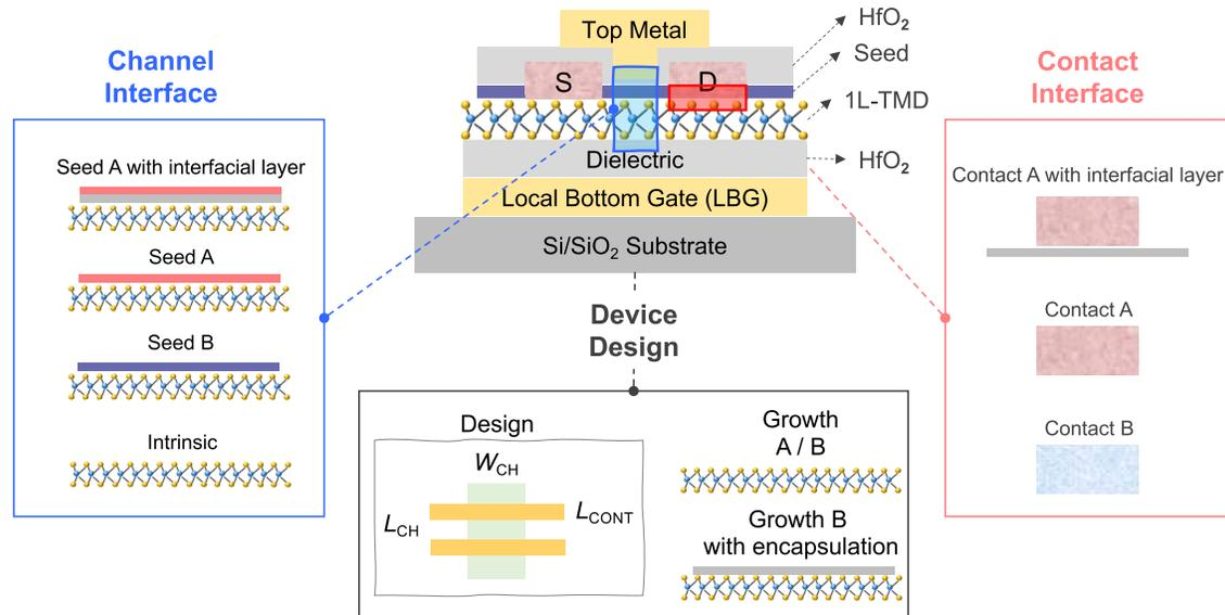
Fig. 1. Features determining the electrical characteristics of 2-D 1L TMD transistors schematic cross section of a 1L-TMD FET with a LBG and a top gate. Various components that govern the device performance are categorized, including the channel region where the top gate-stack is formed, FET device design parameters ( $L_{CH}$ : channel length,  $W_{CH}$ : channel width, and  $L_{CONT}$ : contact length), and the interface between TMD and contact metals.
