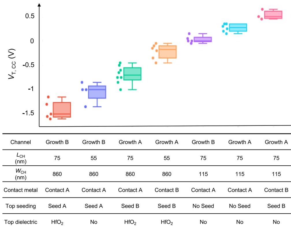
Fig. 6.  $V_{TH}$  tuning through different process combinations. Seven different threshold voltages can be achieved in short-channel 1L-MoS<sub>2</sub> devices, following the recipes predicted by ML optimization of the process conditions and design parameters.
