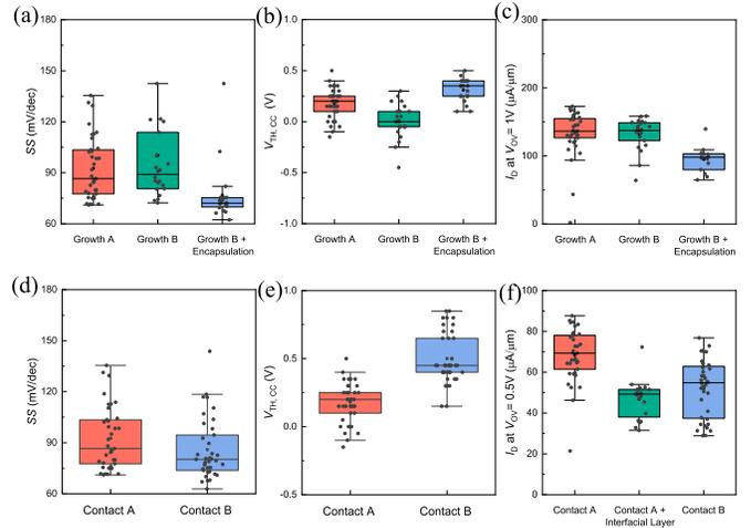
**Fig. 5.** Impact of channel material and metal contact. (a)–(c) Channel material impact. Box plots of (a) SS, (b)  $V_{TH,CC}$ , and (c)  $I_D$  at  $V_{OV} = 1$  V, comparing 1L-MoS<sub>2</sub> grown by MBE, CVD, and CVD with 1L-hBN encapsulation. (d)–(f) Metal contact impact. Box plots of (d) SS, (e)  $V_{TH,CC}$ , and (f)  $I_D$  at  $V_{OV} = 0.5$  V, comparing Ni, Bi, and Ni/1L-hBN contacted 1L-MoS<sub>2</sub> devices.
