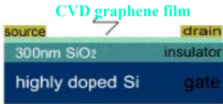
Fig. 3. Schematic cross section of the GFET device made from CVD grown graphitic film transferred to Si/SiO 2 .
