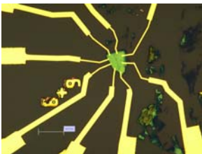
Fig. 7. A small GFET device ("B") made by EBL (scale bar = 34.6 \mu\text{m} ). Black lines on film are wrinkles.
