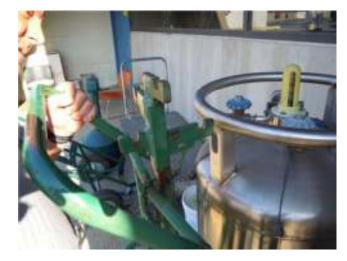
Tip the top of the cart towards the dewar and insert the notch mechanism. Some carts are equipped with a handle to assist with the positioning of the cart.
