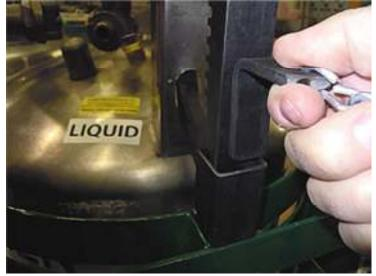
Lean the cart towards the dewar and insert the upward turned hook into the lifting point. Once the hook is fully inserted and snug, the strap can be placed around the dewar and tightened.
