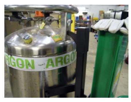
The lifting mechanism is different than the Harper or Anthony carts. The post must be raised as the Barrel Hawk is moved closer to the dewar to fully engage the lifting mechanism with the lifting hole on the dewar. The dewar can now be lifted off the ground by pumping up the hydraulics.
