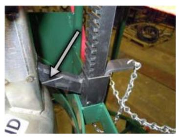
The adjustment of the post is marked on the post. This line on the post (note the white line in the photo) should be even with the top of the hole in the dewar post. The adjustment should be made prior to inserting the post into the dewar lifting hole. The frame of the cart is leaned towards the dewar to insert the post into the lifting hole.
