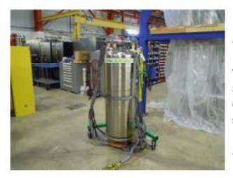
In some cases, when an overhead lift of a dewar is required, a basket sling can be used. The Barrel Hawk is an ideal tool to raise the dewar to install the basket sling. Use the Barrel Hawk to lift the dewar as usual, but do not connect the support straps. Position the basket sling under the dewar and place the webbing and lifting eye on the dewar.
