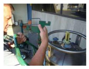
The post must be adjusted for the height of the dewar that is being moved. This mechanism must be lifted up out of the post, rotated, and reinserted into the post.
