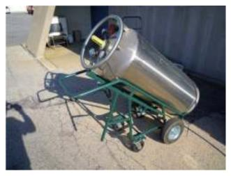
The dewar is now fully tipped and stable on all four wheels. The dewar and cart can now be rolled to the desired location. Check for, and remove, any obstacles that may hinder transport. Be mindful of elevation changes or sloped surfaces.
