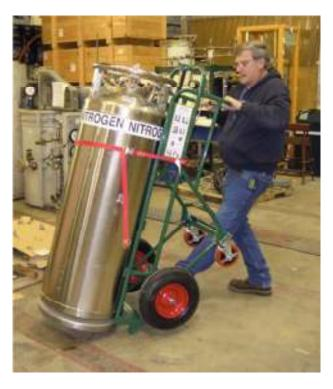
When tilting the cart back, ensure that <u>both hands</u> are on the cart handle(s). <u>Never</u> grab the dewar ring with one of your hands. Place one foot against the lower bar for leverage, and pull back gently using your weight.
