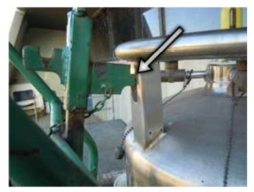
This is a close-up of the desired position of the notched bar. Note that the <u>bottom of the notch is</u> touching the top of the lifting hole on the dewar ring support.
