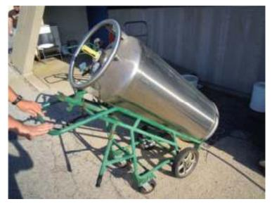
The dewar is now fully tipped and stable on all four wheels. The dewar and cart can now be rolled to the desired location. Check for, and remove, any obstacles that may hinder transport. Be mindful of elevation changes or sloped surfaces.
