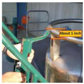
Adjustment of the hook is critical. The post type cart must be adjusted to fit the height of the dewar <u>before</u> the post is inserted in the lifting hole. The correct adjustment is to raise the post so that the top of the lifting post is about one inch higher than the lifting hole.
