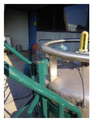
The post should be engaged as in the photo before tipping the dewar back towards you. When the post is fully engaged into the lifting hole, the top of the lifting post is touching the top of the lifting hole. <u>There</u> <u>should be no free play</u>. <u>If the hook does</u> <u>not fit snug, readjust</u>.
