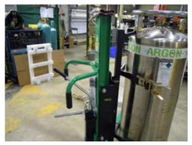
Place the barrel hawk near the dewar. Position the cart's lifting post in line with the lifting hole on the dewar. The lift mechanism is hydraulically actuated.
