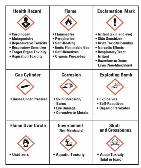
Figure A.VI.1 – Hazard Communication Standard Pictograms
