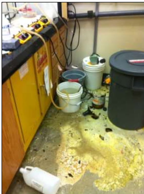
Figure 7.2 – Container Failure Due to Mixing Incompatible Waste Streams
