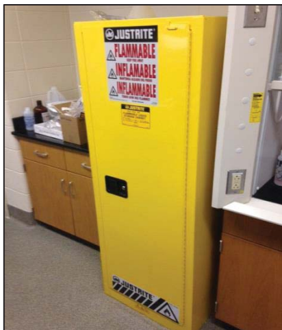
Figure 5.1 – Flammable Storage Cabinet
