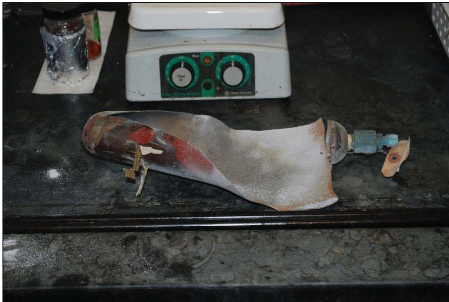
Figure 5.8 – HF Cylinder Incident at Purdue University in 2011
