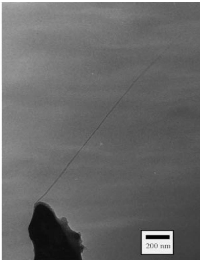
Figure 6.3 Single walled carbon nanotube (SWNT) mounted on a Pt field emitter. The bundle thickness is uneven, with the radius ranging between  $55 \pm 5 \text{ \AA}$  to  $85 \pm 5 \text{ \AA}$ . The end of the bundle is not resolved due to thermal vibrations.
