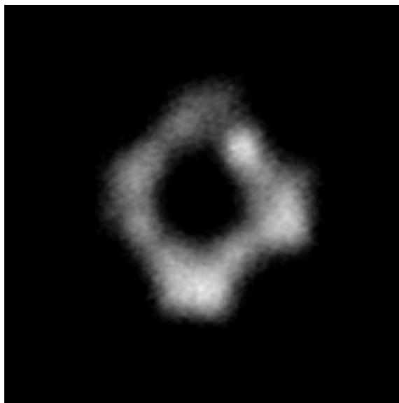
Figure 5.8 Field emission image of a Pt/Ir tip oriented in the 100 direction.
