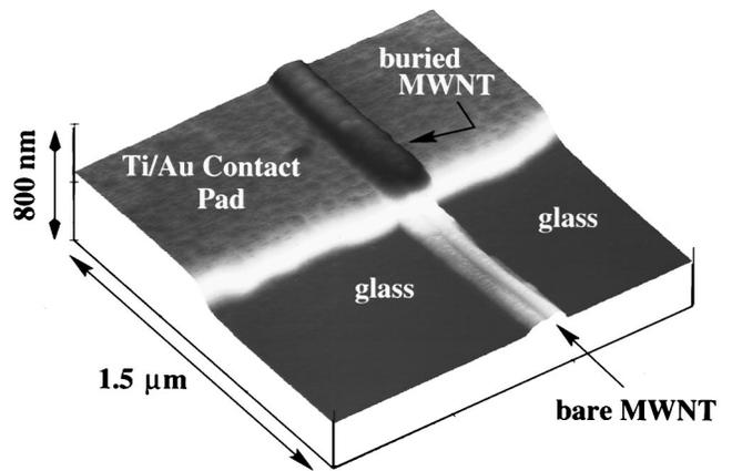
FIG. 2. A 1.5 μm×1.5 μm AFM image of a MWNT (sample No. 4) buried under a Ti/Au contact pad. The image shows the substrate comprised of a glass cover slide, one of the two Ti/Au contact pads, a section of the MWNT buried under the Ti/Au film, and a section of the bare MWNT which emerges from under the Ti/Au contact pad.
