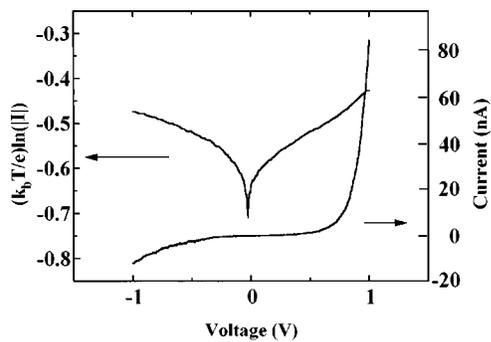
FIG. 4.  $I(V)$  data from a MWNT (sample 3) showing diode-like conduction. The minimum diameter of this tube as determined from AFM studies is  $\sim 130$  nm. The length of this tube between the contact pads is  $\sim 4$   $\mu\text{m}$ . The forward bias can be fit to a standard diode equation  $I = I_0 e^{e\phi/kT} e^{eV/\eta kT}$ . A plot of  $(k_B T/e) \ln(|I|)$  vs  $V$  is also provided and yields an ideality factor  $\eta \approx 5.6$ .
