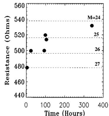
FIG. 3. A plot of resistance vs time (after the initial measurement of resistance) for a highly linear MWNT (sample 4). The tube resistance is found to abruptly change with time. The horizontal dotted lines represent quantized resistance values of  $M/G_0$ , with  $M=24, 25, 26,$  and  $27$ . The diameter of this tube as determined from AFM studies is ~40 nm. The length of this tube between the contact pads is ~4 μm.
