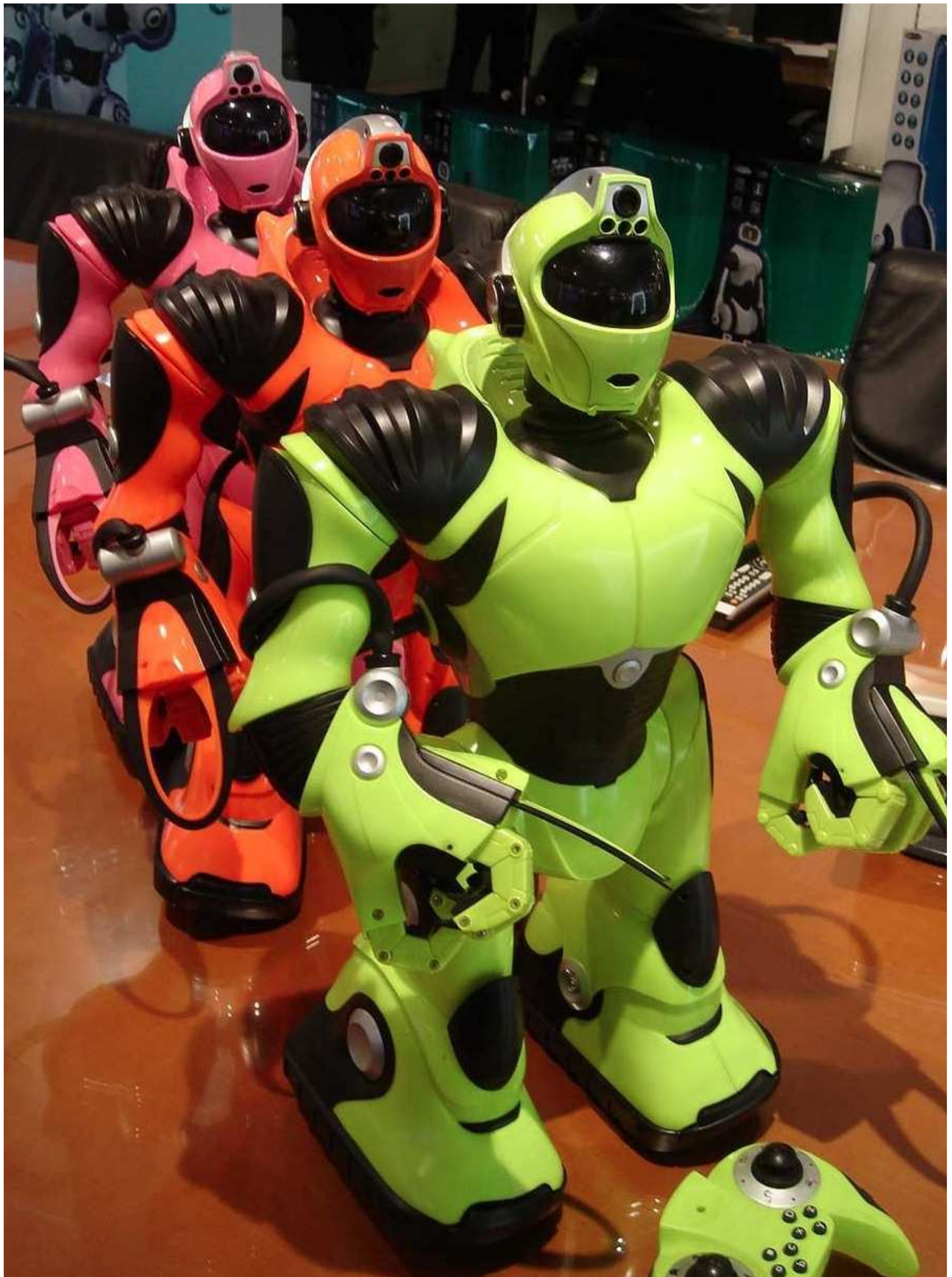
Figure 6 The Robosapien Version 2 (RS2) was a 13 motor, 2 foot high fully controllable humanoid robot with full-sized hands and multi-function remote. Now a collectors' item, it was designed to be fully hackable with
