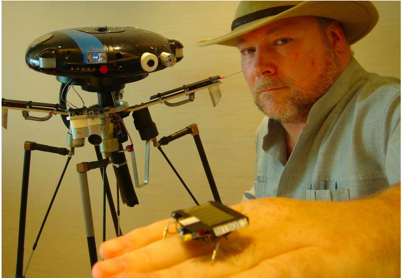
Figure 3 Tilden poses with his five-foot-high spider robot "Roswell", and the inch long solar-powered "Bitbot", both held together with more springs than bolts. (SOURCE: Mark W. Tilden)
