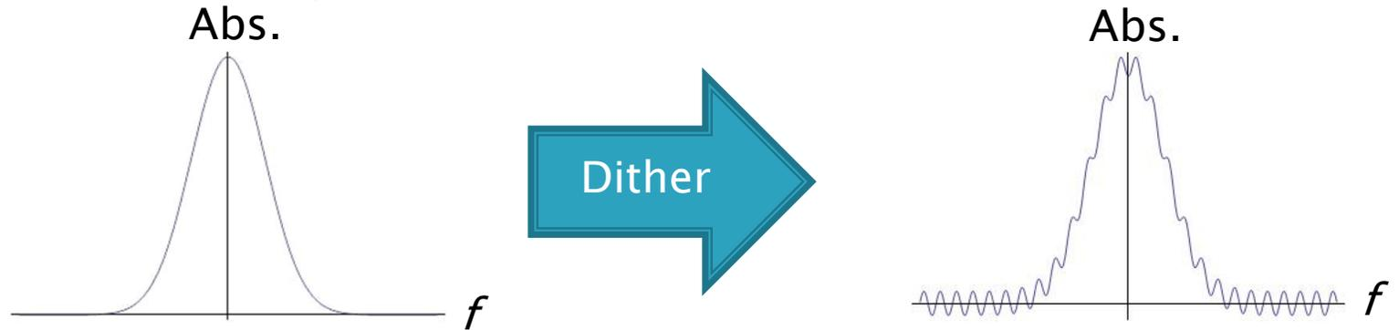
2. Use a lock-in amplifier and low-pass filter to convert amplitude of dither on signal to voltage
