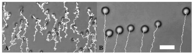
**Figure** 3 - A) Tracks for 2 micron beads on a tilted microscope stage also show directed motion due to gravity, but a much larger contribution from Brownian motion (due to the smaller size). B) Silica bead trajectories after tilting the microscope. This motion has both a random (Brownian) component as well as directed (coherent) motion due to gravity.
