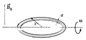
is a uniform magnetic field B perpendicular to the rotation axis. Assume the conductivity of copper is  $\sigma$ , the density is  $\rho$ , and neglect self-inductance. Calculate the decay time for the rotational frequency to decrease to 1/e of its original value  $\omega_0$ , assuming all loss is due to resistive heating.
