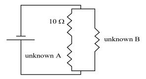
You should try to set up this circuit yourself. However, if you need a little help, you may refer to the diagram below. In fact, it is a combination of resistors in parallel and in series.
