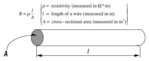
In the equation above, the <u>resistivity</u> of a material  $\rho$  is just a constant of proportionality, which relates length and area directly to the resistance *R*. This resistivity depends only on the type of the material and has no dependence on geometry.
