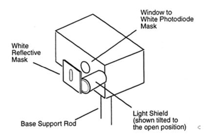
1.13. **Close the "Light Shield"**. Then, **press** the red "PUSH TO ZERO" button on the side panel of the photocell box to discharge any accumulated potential in the unit's electronics. This will assure that the apparatus records only the potential due to the light shining on the
