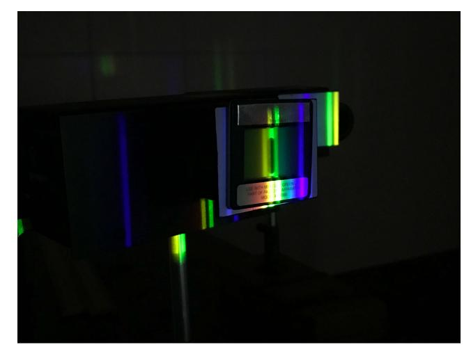
1.11. The diffraction grating creates two first-order patterns. One on the left side of the white, undiffracted line and one on the right side.
