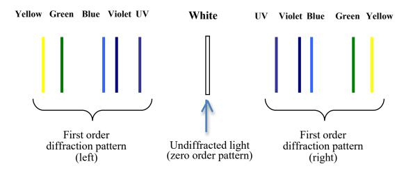
The second order patterns are also visible and they are located further away from the undiffracted white line. The order of colors for the second order pattern is the same as for the first order pattern.
