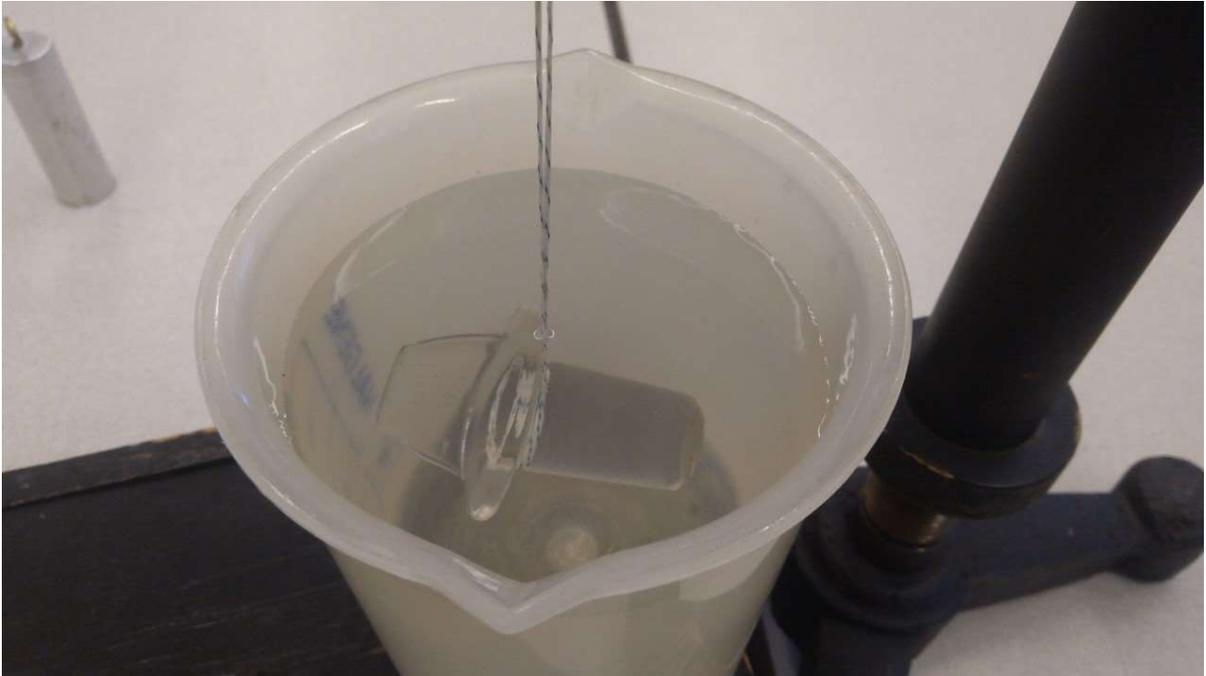
Take two tension measurements, one when the glass is in air and one while the glass is submerged in the water and use the formula to calculate the glass piece's volume.
