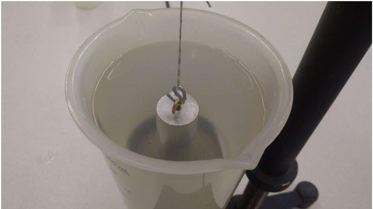
Using the Archimedes' principle, calculate the density ( $\rho$ ) for the measured aluminum cylinder (Equation 3). Compare this result with the known value ( $\rho_{\text{aluminum}} = 2700 \text{ kg/m}^3$ ). What is the percent difference?
