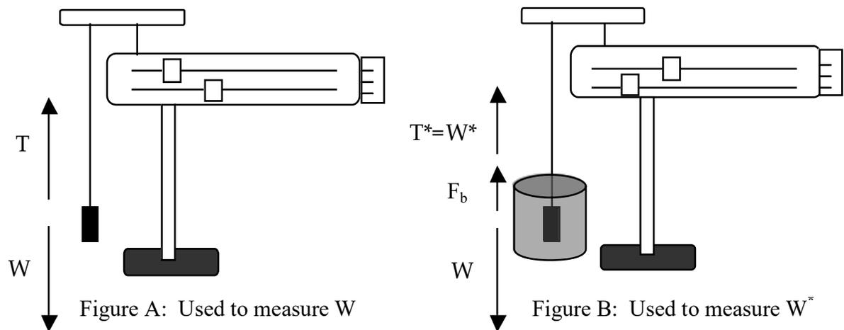
In Figure A, the tension ( $T$ ) in the string is equal to the **weight ( $W$ )** of the object and is measured by adjusting the two sliding bars until the balance is centered.  $T = W = mg$ .
