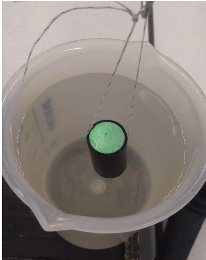
Determine the percent composition of this cylinder by finding the weight of the two-metal cylinder while the cylinder is in air and then again when it is submerged in water.
