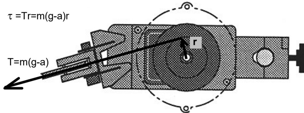
Fig. 2. Adjustment for clamp-on Super Pulley<sup>1</sup>
