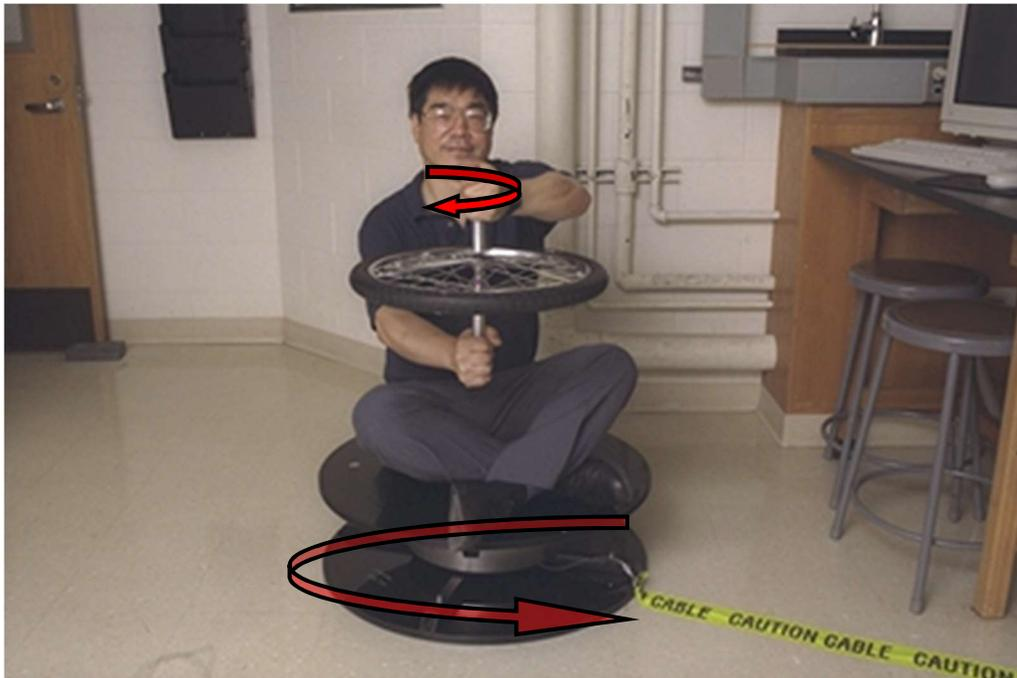
When the person on the platform is finished, slow and then stop the platform. Take the wheel from the person and hold the platform steady while the person gets off the platform.
