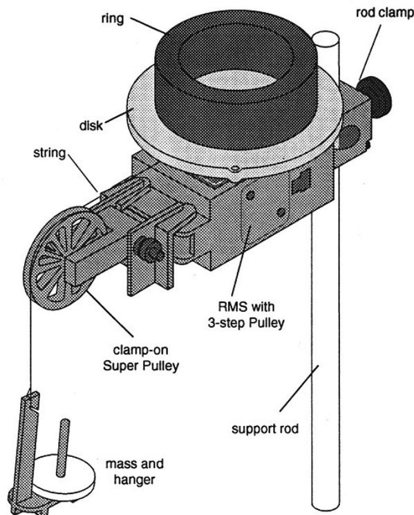
Fig. 1. Rotational inertia setup of disk and ring
