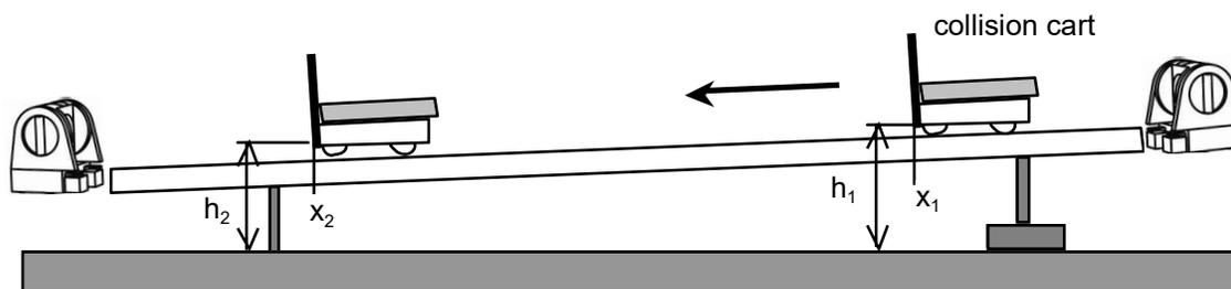
Figure 2. Illustration of position and height measurements on track.
