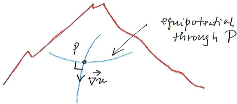
Consider a mountain where we characterize each point by a gravitational potential energy  $u(P=x, y, z)$ . Then  $\vec{\nabla}u(P)$  points along the fall line which is the path of steepest descent. If a ski came loose, this is the path it would take.
