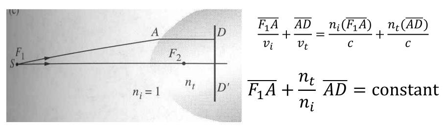
• This is the equation for a hyperbola if  $n_t/n_i > 1$  and the equation for an ellipse if  $n_t/n_i < 1$ .
