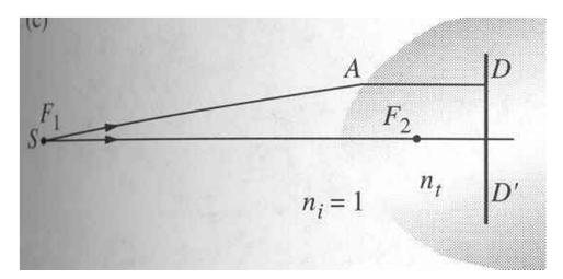
• Time to travel from S to plane DD' must be equal for all points A on the surface.
