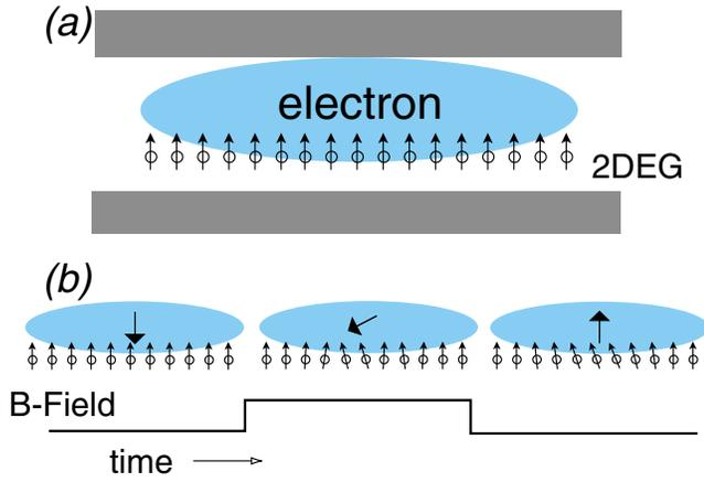
FIG. 1 (color online). (a) A schematic of an electron trapped in a quantum dot with polarized nuclei. (b) Storage, where a pulse in the magnetic field starts and brings the spins into resonance for a  $\pi$  pulse. Readout is the same process in reverse.
