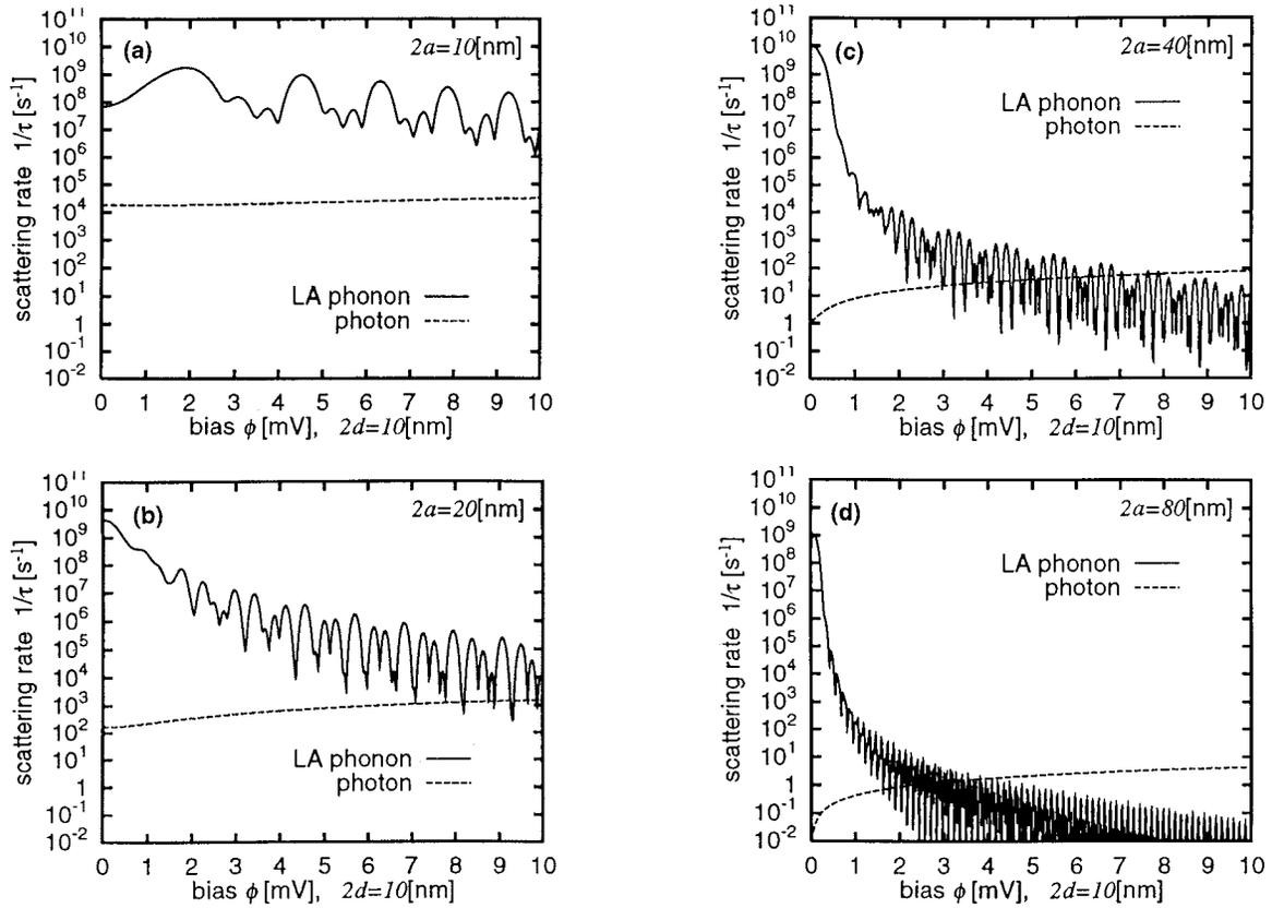
FIG. 6. The electron scattering rate at  $T=0$  K due to emission of LA phonons or photons in CQDs where the distance between QDs is  $2d=10$  nm and (a) the side of a QD is  $2a=10$  nm, (b)  $2a=20$  nm, (c)  $2a=40$  nm and (d)  $2a=80$  nm.  $\phi$  denotes the bias voltage applied between QDs.
