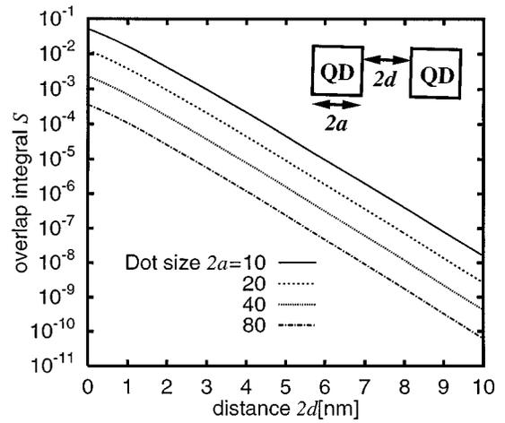
FIG. 4. Structure dependence of the overlapping integral  $S$  for the InAs/AlSb system.  $2a$  and  $2d$  denote the side of a QD and the distance between the different QDs, respectively.
