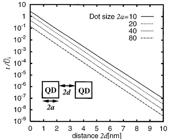
FIG. 5. Structure dependence of the ratio of the transfer energy  $t$  to Coulomb energy  $\tilde{U}_i$  for the InAs/AlSb system.  $2a$  and  $2d$  denote the side of a QD and the distance between the different QDs, respectively.
