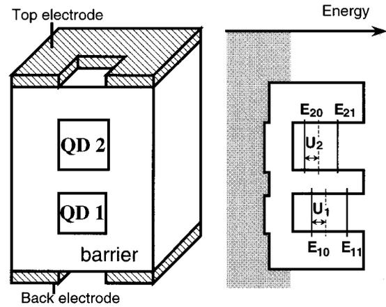
FIG. 1. The cross section of the device structure and energy diagram of the device when no bias is applied.
