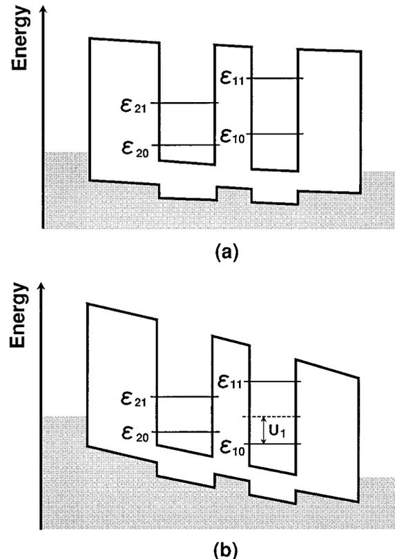
FIG. 2. The arrangement of the energy levels (a) when the first bit of information is input and (b) when the second bit of information is input.
