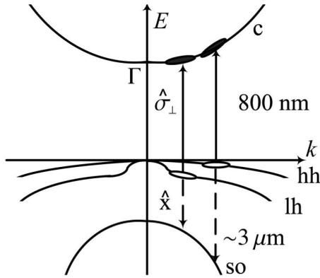
FIG. 1. The femtosecond output of a Ti:sapphire laser at  $\lambda_{\text{pump}} = 800$  nm (solid line) generates oriented holes in the hh and lh. The change in the degree of circular polarization of a transmitted, time-delayed  $\lambda_{\text{pr}} \sim 3 \mu\text{m}$  synchronized probe pulse (dashed line) corresponding to the so-hh and so-lh transitions is proportional to the spin state at that value of the delay.
