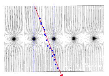
**Typical parameters:** L=5mm, d=1mm,a<sub>wire</sub>=20mm.
