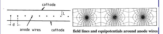
Capacitive coupling of non-screened parallel wires? Negative signals on all wires? Compensated by positive signal induction from ion avalanche.
