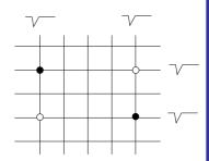
Charge division. Resistive wires (Carbon,2kΩ/m).
