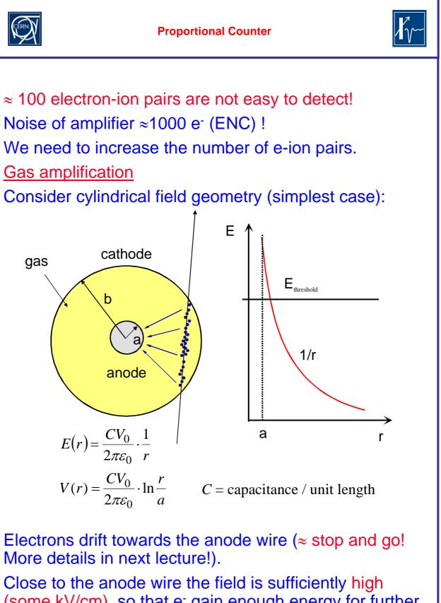
(some kV/cm), so that e<sup>-</sup> gain enough energy for further ionization  $\rightarrow$  <u>exponential increase</u> of number of e<sup>-</sup>-ion pairs.
