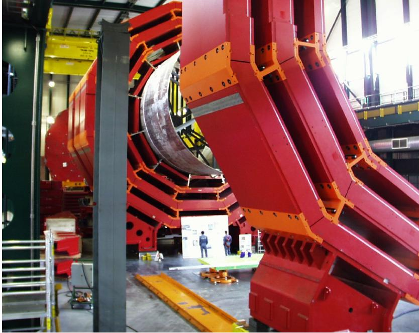
Figure 10: A view of the yoke at an early stage of magnet assembly at SX5. The central barrel supports the vacuum chamber of the superconducting coil. At the rear, one of the closing end cap disks is visible.
