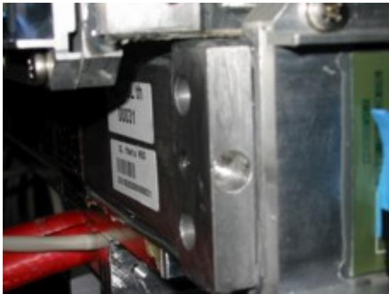
Figure 143: Corner blocks of an SL. These pieces also carry the reference marks with respect to which the wire positions are measured.
