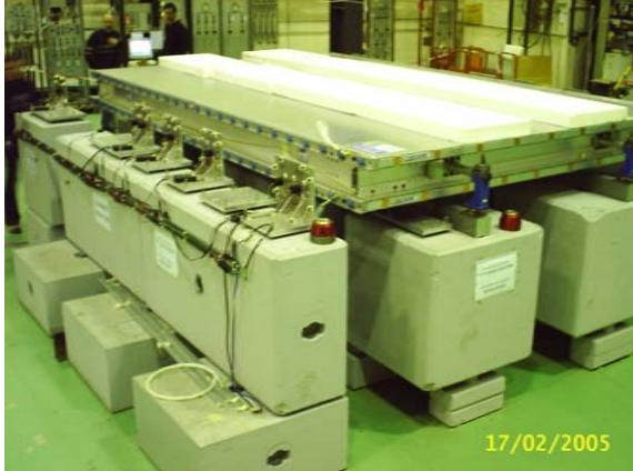
Figure 156: The chamber calibration bench in the CERN ISR Lab.
