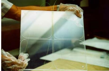
Figure 115: View of a typical tile of HO with WLS fibres inserted in the 4 grooves of the tile.
