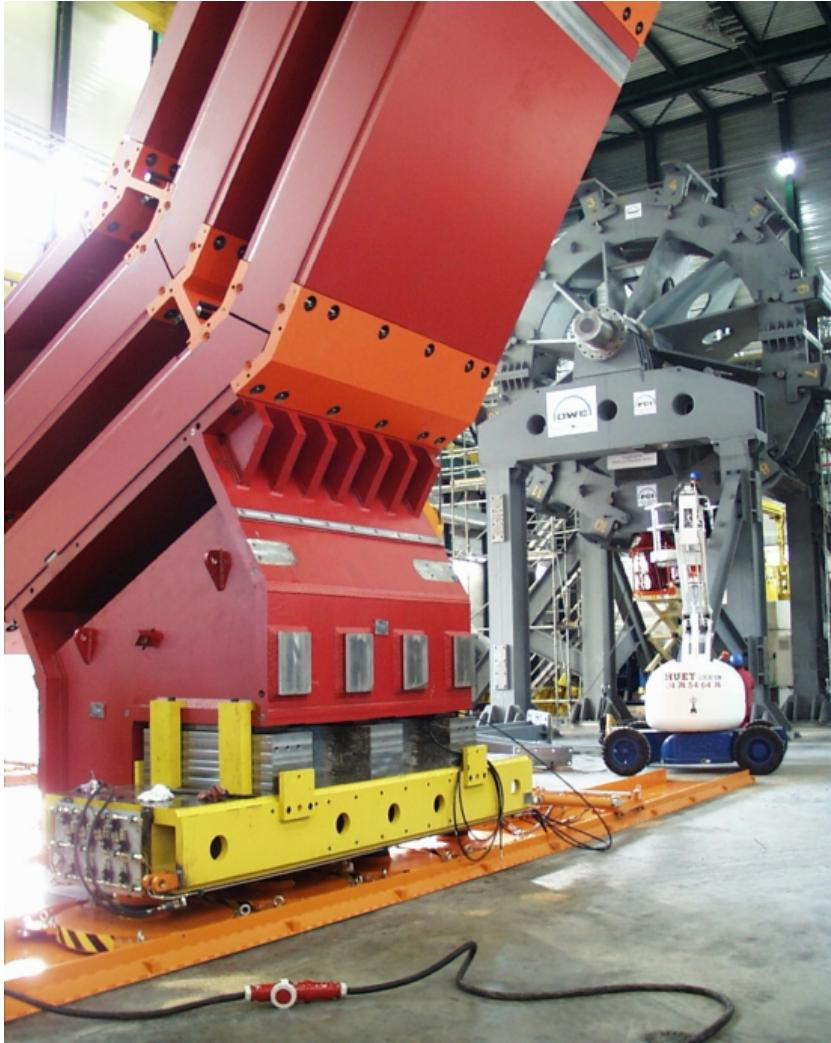
Figure 252: A transport beam for barrel rings with 4 air pads fixed on it.
