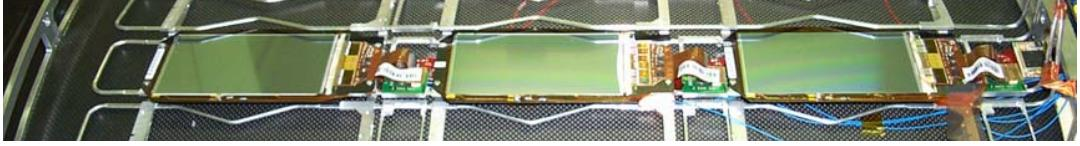
Figure 54: Three TIB modules mounted on a layer 3 shell. The Kapton mother cable runs underneath. A CCUM module at the end of the string interfaces the modules to the control ring. Also visible are the three analog opto-hybrids (see text) and fibers.
