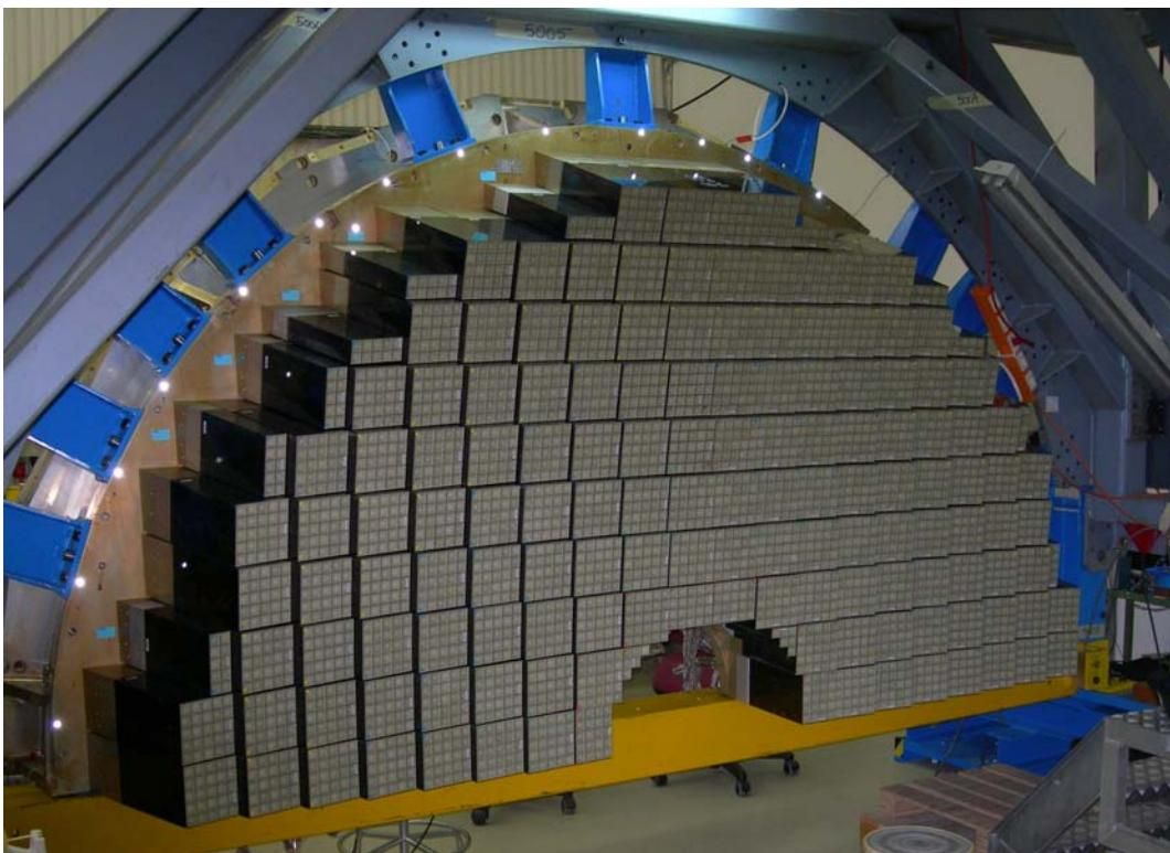
Figure 77: An endcap Dee, fully equipped with supercrystals.
