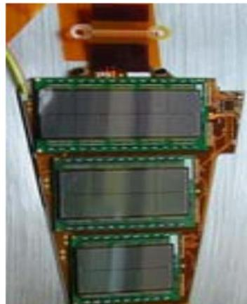
Figure 46: Sketches of the two types of FPix panels showing the different sizes and numbers of the plaquettes on each (left side). A photograph of an actual 3-plaquette panel (right side).
