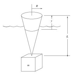
(a) Calculate the volume of water displaced when the top of the float is located a distance y above the surface of the water.
