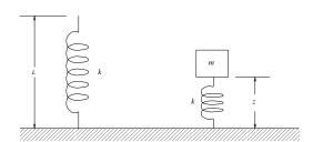
(a) The weight of the mass compresses the spring. What will be the compressed length of the spring,  $z_0$ , when the mass is in equilibrium?
