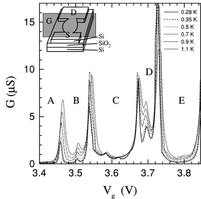
FIG. 1. Differential conductance  $G$  in the quantum dot as a function of the gate voltage  $V_g$  at six different temperatures. The  $G$  is measured with  $10 \mu\text{V}$  ac source-drain bias at a frequency 7.7 Hz, zero dc bias and  $B = 0$ . Letters A . . . E label Coulomb blockade valleys. Schematic of the device is shown in the inset. Poly-Si gate (G) covers the dot and adjacent regions of source (S) and drain (D).
