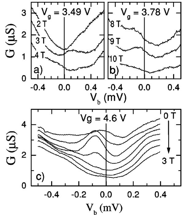
FIG. 4. Differential conductance  $G$  as a function of dc bias  $V_b$  in three different Coulomb blockade valleys. In these valleys, peaks in  $G$  are observed at  $B \neq 0$ . Curves are offset by  $0.5 \mu\text{S}$  in (a) and (b) and by  $0.25 \mu\text{S}$  in (c), except for the bottom curves in each plot.
