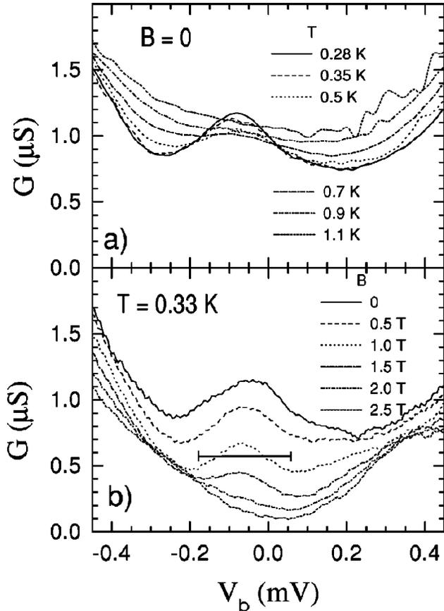
FIG. 2. Differential conductance  $G$  as a function of a dc source-drain bias  $V_b$  at different (a) temperatures, and (b) magnetic fields at a fixed gate voltage  $V_g = 3.57$  V. The (a) and (b) data sets were taken one day apart, which resulted in a small difference between  $T = 0.35$  K data in (a) and  $B = 0$  data in (b). The bar in (b) indicates twice the Zeeman energy  $2E_Z = 2g\mu_B B = 0.23$  meV ( $g = 2$ ) at  $B = 1$  T.
