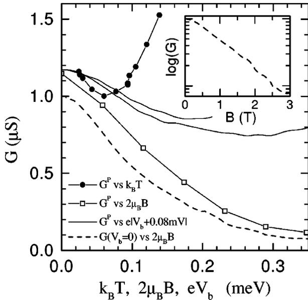
FIG. 3. Peak differential conductance  $G^P$  at  $V_b = -0.08$  mV is plotted as a function of temperature  $k_B T$  at  $B=0$  ( $\bullet$ ), magnetic field  $2\mu_B B$  at  $T=0.3$  K ( $\square$ ). The two solid curves are  $G^P$  vs bias  $e|V_b - V_b^P|$  at  $B=0$  and  $T=0.28$  K, where  $V_b^P = -0.08$  mV is the peak position. Dashed line is  $G$  vs  $B$  at  $V_b=0$  and  $T=0.3$  K. Inset:  $G$  at  $V_b=0$  falls almost exponentially as a function of  $B$ .
