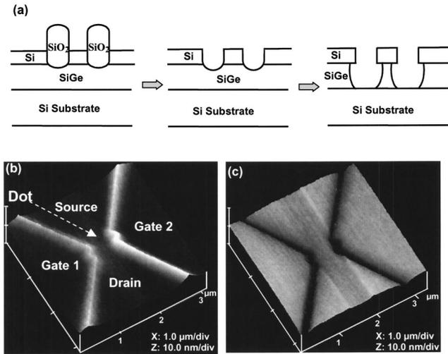
FIG. 2. (a) Process to pattern Si/SiGe nanostructures: AFM oxidation on the Si cap; HF dip to remove SiO<sub>2</sub>; and wet selective etching to pattern the SiGe layer. (b), (c) AFM images of a SiGe quantum dot fabricated by this nanopatterning approach after AFM oxidation and selective wet etching, respectively.
