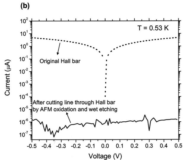
FIG. 3. (a) AFM image of a line cut across the Hall bar by AFM oxidation and selective wet etching. The sample was pre-patterned by optical lithography and RIE to create a mesa with Hall bar structure. (b) Hall bar resistance measurement at  $T = 0.53$  K before and after cutting a line across the Hall bar.
