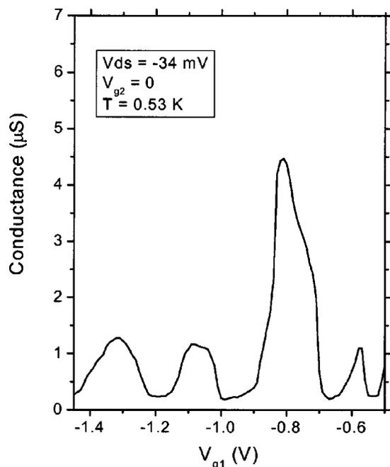
FIG. 4. Electrical characteristics (conductance vs gate voltage) of a SiGe quantum dot fabricated by AFM oxidation and selective wet etching that exhibits Coulomb blockade oscillation at  $V_{ds} = -34$  mV and  $T = 0.53$  K.
