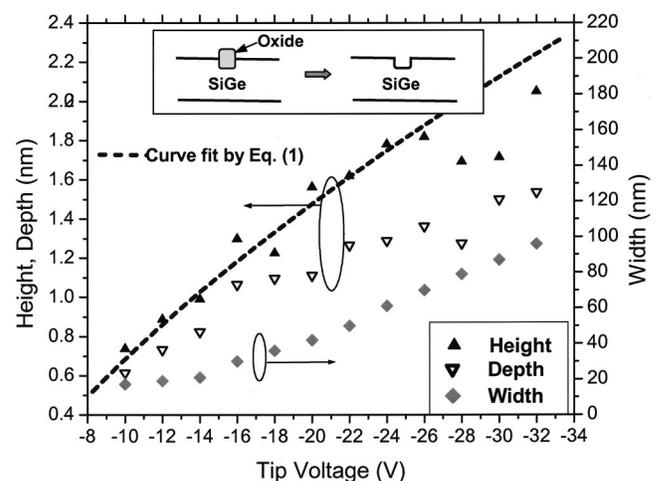
FIG. 1. Height, depth (after HF etching) and FWHM of AFM oxidation lines on strained Si<sub>0.8</sub>Ge<sub>0.2</sub> alloys as a function of different bias voltages between the tip and sample. The writing speed was 1.6  $\mu\text{m/s}$ . The dashed line is a fit of the height data using Eq. (1). The inset is a schematic of AFM oxidation and oxide removal.
