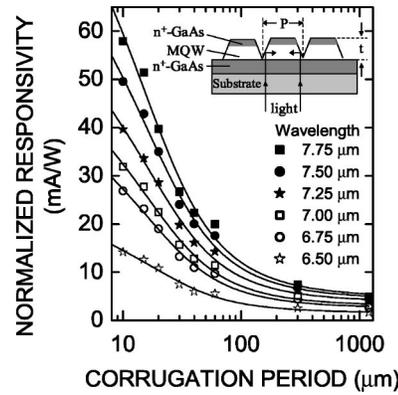
FIG. 3. Normalized responsivity  $NR$  of C-QWIPs as a function of C-QWIP period  $P$  for different wavelengths. Symbols: Experimental data at 10 K for voltage bias  $V_b = 6$  V. Lines: least-squares fit of Eq. (1) to the data. Inset: side-view of a C-QWIP with three corrugations. The rays inside the C-QWIP show back illuminated normal incidence light undergoing total internal reflection at the sidewalls to get coupled to the intersubband transitions in the quantum wells.
