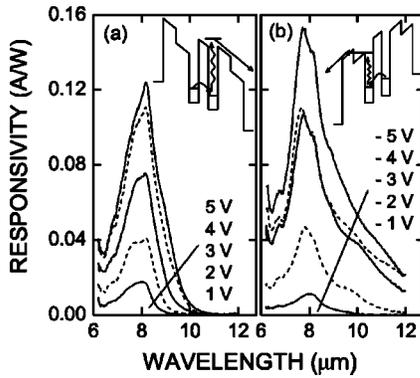
FIG. 1. Spectral responsivity  $R$  of  $45^\circ$ -edge coupling QWIP measured at 10 K for (a) positive and (b) negative bias  $V_b$ . For both (a) and (b),  $|V_b| = 1, 2, 3, 4,$  and  $5$  V for the bottom to the top curve. Inset: Conduction band diagram and photoexcitation mechanism of two-color QWIP based on coupled QWs for (a) positive and (b) negative  $V_b$ .
