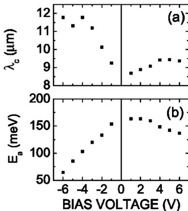
FIG. 2. Bias  $V_b$  dependence of (a) cutoff wavelength  $\lambda_c$  and (b) electron activation energy  $E_a$  of two-color QWIP.  $\lambda_c$  is obtained from Fig. 1 using  $R(\lambda_c) = 0.2 \times R(\lambda_p)$ , where  $\lambda_p$  is the peak wavelength.  $E_a$  is extracted from the temperature dependence of dark current.
