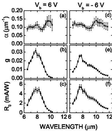
FIG. 4. Wavelength dependence of absorption coefficient  $\alpha$ : (a) and (d), gain  $g$ : (b) and (e), and  $R_0$ : (c) and (f) for bias voltage  $V_b = 6$  V and  $-6$  V, respectively.  $\alpha$ ,  $g$ , and  $R_0$  are extracted from fitting Eq. (1) to normalized responsivity data.
