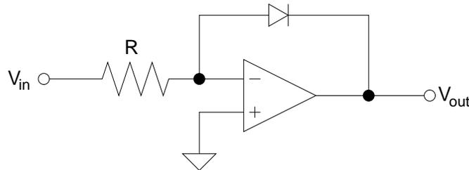
4. Determine the relation between  $V_{out}$  and  $V_{in}$  in the following *exponential amplifier* op-amp configuration:
