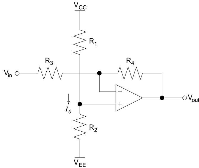
As a constraint, suppose that the current used by the voltage divider between  $V_{CC}$  and  $V_{EE}$  specified to be  $I_0$ .
