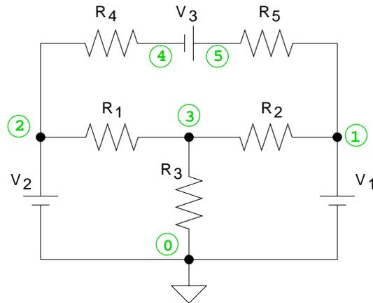
(a) Assign currents  $I_1$ ,  $I_2$  and  $I_3$  flowing *clockwise* through the three loops containing voltage sources  $V_1$ ,  $V_2$  and  $V_3$ , respectively. Then write the  $3 \times 3$  matrix equation that relate the currents, resistances and voltage sources. You do not need to solve this system of equations.
