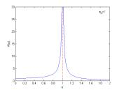
Amplitude gets very large when the frequency of the driving force is close to the natural oscillation frequency.
