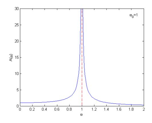
Amplitude gets very large when the frequency of the driving force is close to the natural oscillation frequency.
