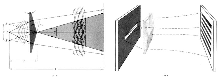
The general approach with many interference problems is to figure out how a particular system is equivalent to a double-slit experiment.
