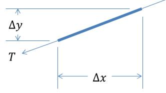
Work needed to stretch the string in the vertical direction:
