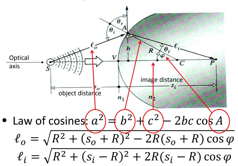
Fermat's principle: Light will travel on paths for which the optical path length is stationary (ie, minimal, but possibly maximal)
