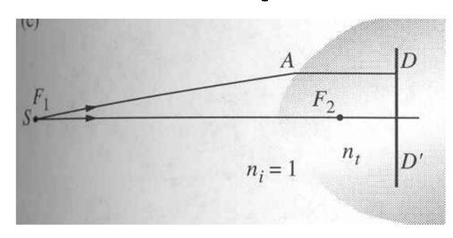
$$\frac{\overline{F_1 A}}{v_i} + \frac{\overline{AD}}{v_t} = \frac{n_i(\overline{F_1 A})}{c} + \frac{n_t(\overline{AD})}{c}$$
