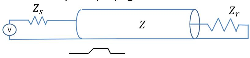
The system is linear, so the observed signal at any point is the sum of all incident and reflected waves.
