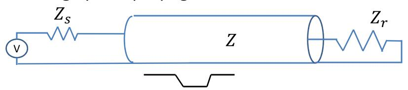
The pulse can also be reflected from an impedance mismatch at the source:
